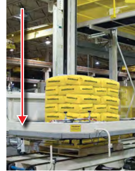
The shrink frame is lowered and raised to evenly shrink the entire hood over the load.
