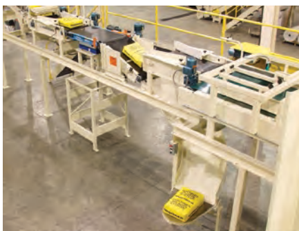
Automatic reject station kicks out under and overweight bags.
