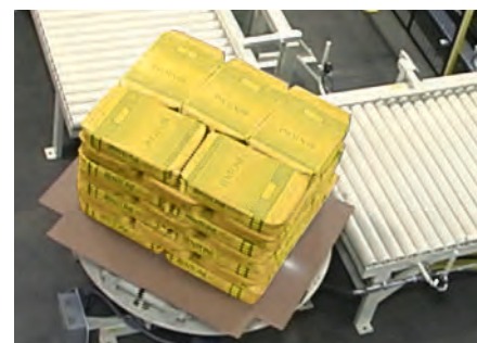
Heavy-duty turntable live roller with all rollers chain driven.
