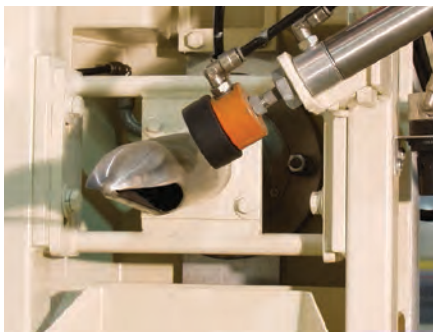
Nozzle with bag detection device.
