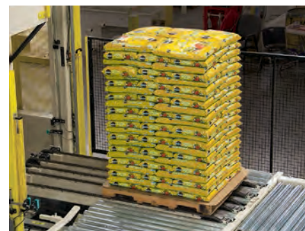
Roller/chain transfer for proper load flow orientation.
