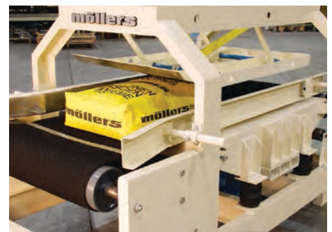
Bag equalizer flattens air-tight, sealed bags.
