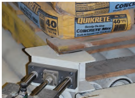
Pallet lock feature secures the pallet during stacking.
