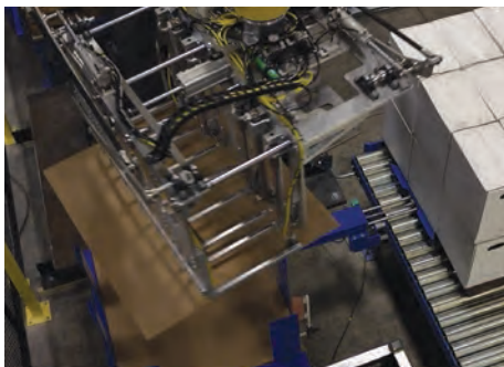
Robotic arm positions tie-sheets between layers to improve load stability.
