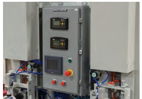
Independent control of each filling spout ensures accurate weight tolerances.
