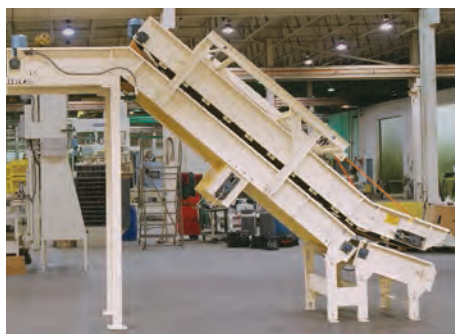
Bag flattener elevator flattens and elevates bags in reduced floor space.
