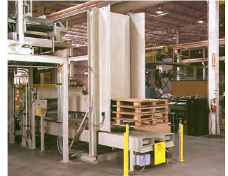
The standard empty pallet magazine holds 20 empty pallets.
