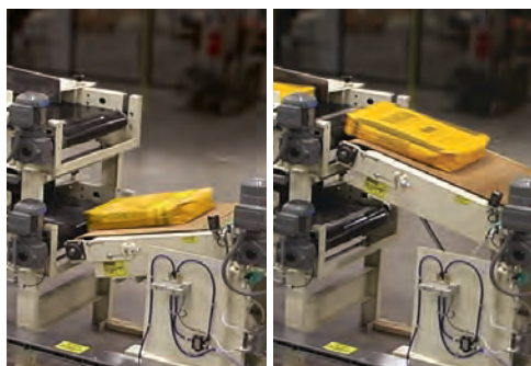
A pivoting conveyor feeds accumulated product from multiple lines into the dual stacking palletizer.
