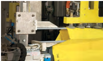
Conveyorized bag feeder provides a steady supply of bags to the placer.
