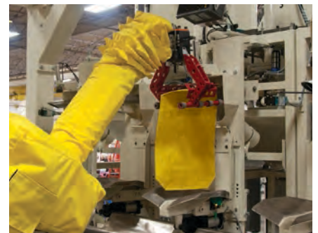
An optional pressurized suit is available to accommodate different environmental area requirements.
