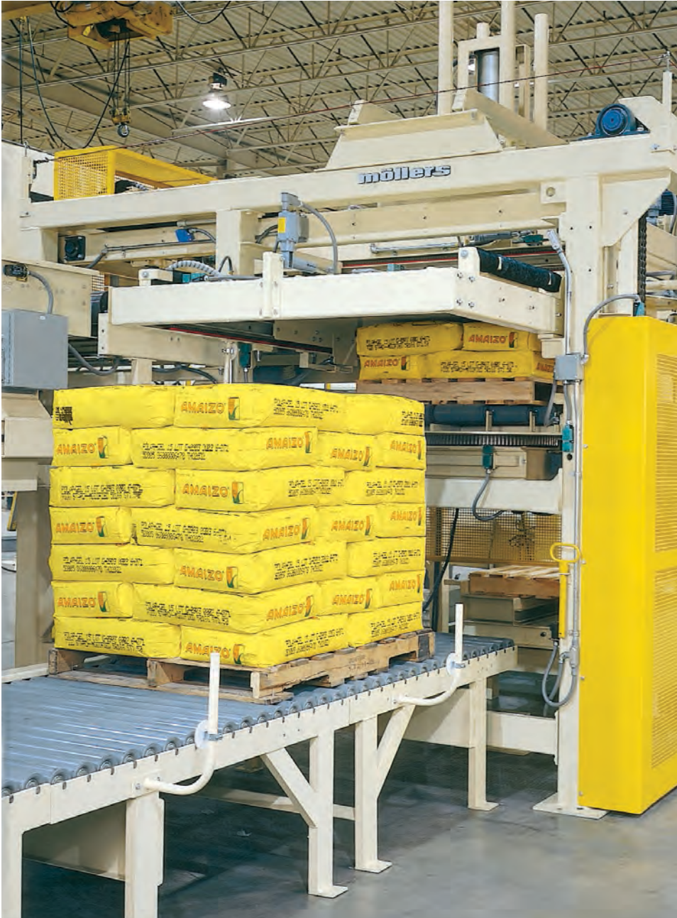
The standard empty pallet magazine holds 20 empty pallets.
