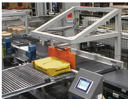
Side reject station automatically removes bags that do not meet proper tolerances.
