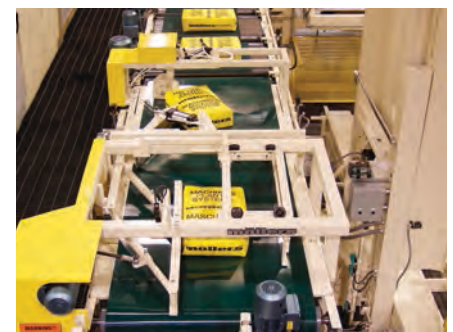
Bag turning post handles up to 50 bags per minute.
