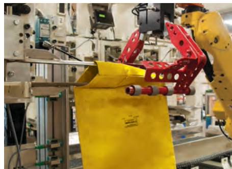
The robotic arm secures the bags from the duck-bill while maintaining open valve position during transition to filling spout.
